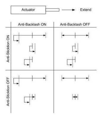
For each setting scenario, the starting position is denoted by the solid vertical line and the final position is denoted by the dotted vertical line. There are four possible moves for each scenario: long move positive, long move negative, short move positive and short move negative. The arrows show the path that would be traversed for each scenario.
